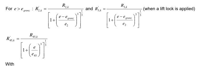
e ... Distance between midplane of beam hanger and support axis of main beam (or rather column axis) in m. For e > 0,2 m additional arrangements for limiting moment interaction need to be done.
